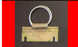
This metal arming key prevented contact between the batteries and the transmitter prior to launch.
